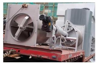
fish and remove the floating objects and sediments at the water intake, squeeze the grid slag dry and drain it after dehydration.
