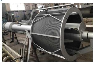
and there are nylon brushes and flushing water nozzles above the drum, The grid slag is removed, dried and dehydrated by screw conveying operation, transported to the upper discharge hopper and transported away by conveyor.
